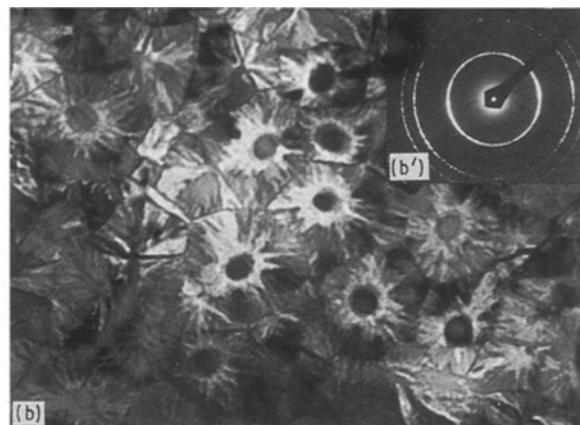
Figure 15 Segregated microstructures in Co–Cr films deposited at a T_s of 140 °C and P_{Ar} adjusted to (a) 3.999, (b) 1.333, and (c) 0.5332 Pa.
